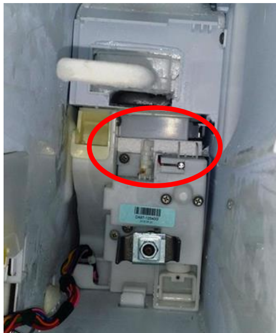
Auger Fan Blocked by Styrofoam
